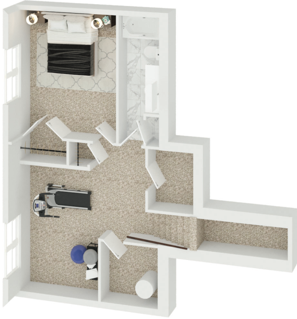
BASEMENT FLOOR PLAN Ceiling Height: 8'-11"
