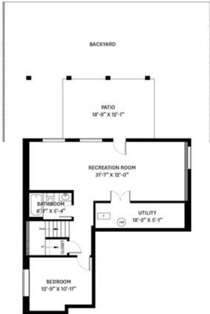
LOWER FLOOR PLAN Ceiling Height: 7'-11"
