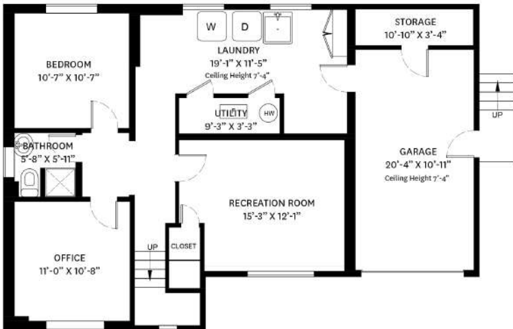
LOWER FLOOR PLAN Ceiling Height: 7'-6"
