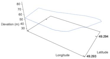
Max Elevation: 59.40 m | Min Elevation: 49.39 m | Difference: 10.01 m  $\,$
